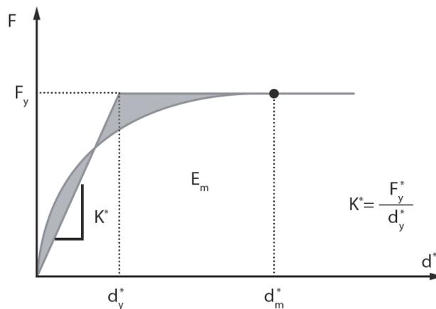
Figure 1: Linearization of the capacity curve[18]
