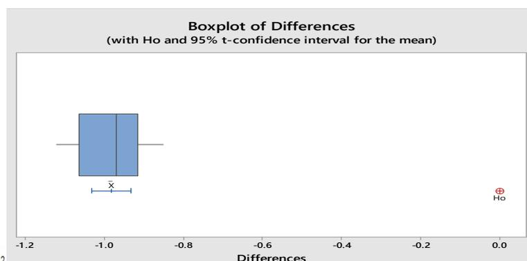
**Paired T-Test and CI: Before, After for Shaping**
