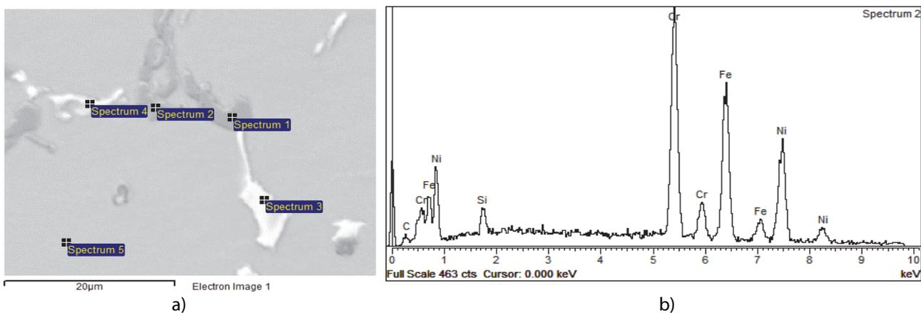
Figure 2 Micrograph of present phases in as-cast HP40 Nb alloy: a) SEM micrographs (BSE), b) EDS spectrum of  $M_7C_3$  carbide (M = Cr, Ni, Fe) in examination point 2 (Spectrum 2)
