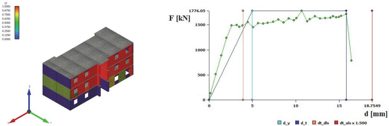
Figure 6: (left) Damage factor  $CF$ , (right) pushover force-displacement curve with idealized bilinear force-displacement diagram for the model M3, +X direction and uniformly distributed load
