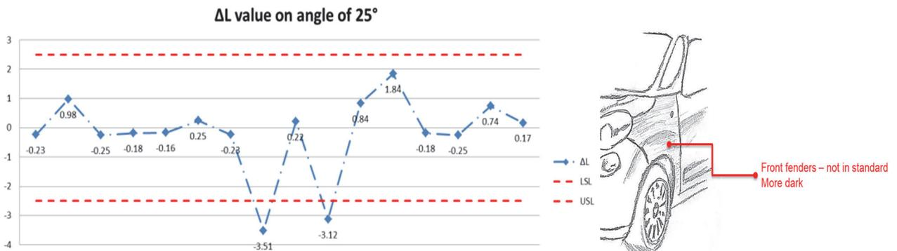
Figure 9: The results of measurement of the entire product after color modification.
