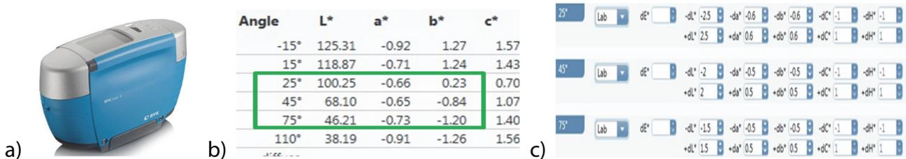
Figure 2: A new method certification of color harmony on a vehicle (a) - measuring device "BYC MAC", b) - measured values, c) – defined standards [12].
