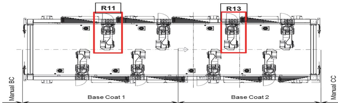
Figure 10: The position of the robot R11 and R13 within the automatic painting process.
